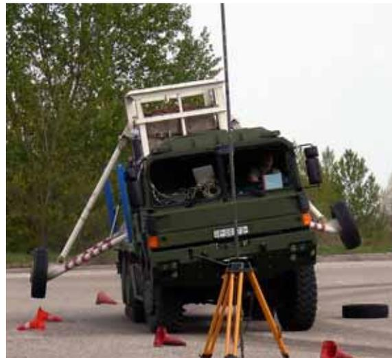
In the frame of the project we tested the applicability of the standard of safety critical electronic systems (IEC 61508) in case of an electronically controlled braking system. The regulation of ECE R13 as a special requirement of the vehicle sector prejudices the application of IEC standard in case of the several function of the braking system. We analysed the aspects of partial or full changing of the control functions from the pneumatic to the electronic one in
